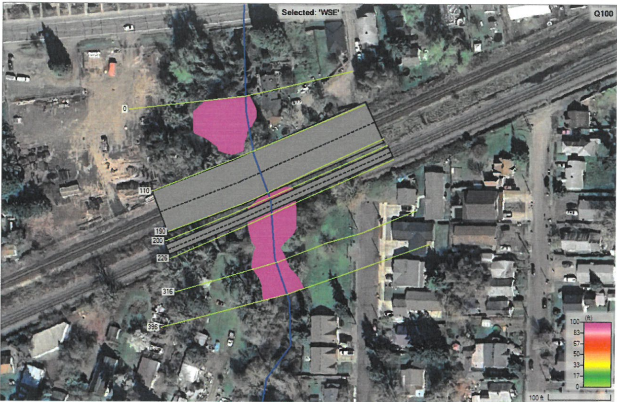
Plan View of Modeled Reach - 100-year Floodplain with Proposed Conditions
